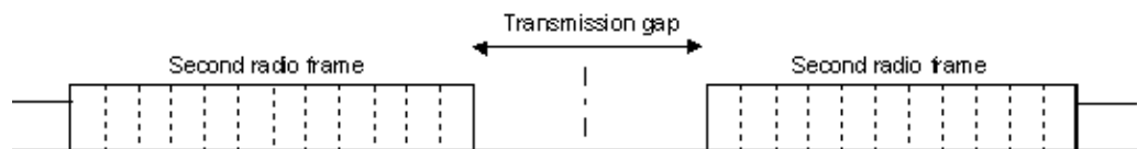
Fig. 5-14: Envelope of compressed mode signal with double-frame method
